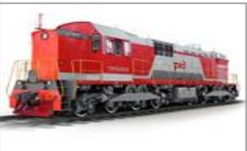
TEM7A 8-axle shunting & clean-up locomotive, 1470 kW
