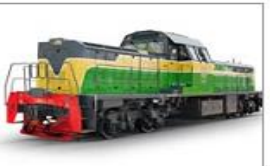
TEM9H shunting locomotive with hybrid drive, 880 kW
