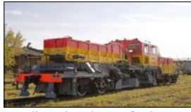
Ballast distributor & planner "RPB"
