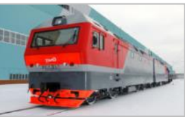
ZE56 two-piece cargo DC locomotive
