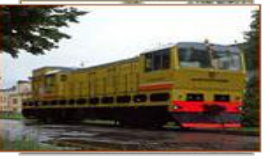
Track rail welding self-powered machine "PRSM"
