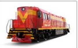
TEM9, TEM9TA 4-axle shunting locomotive, 880 kW
