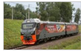
ZE57 AC locomotive with asynchronous traction motors
