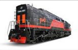
TEM14 8-axle two-diesel shunting & clean-up locomotive, 1,800 kW
