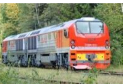
TG16M Two-piece mainline locomotive, 2,940 kW
