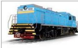
TGM4B 4-axle shunting locomotive, 588 kW
