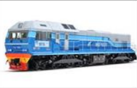
TE8 8-axle locomotive of mainline type, 2,200 kW
