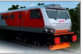
TE35 Mainline single-section locomotive, 3,700-4,200 kW
