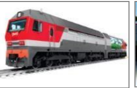
GT1h Mainline gas turbine carrying train, 8,500 kW
