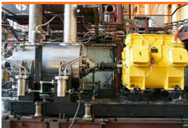
Multi-stage centrifugal horizontal sectional and double casing pumps
