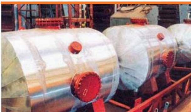
Steam separation unit for Verkhne-Mutnovskaya Geothermal Power Plant
