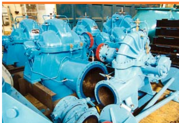
Horizontal centrifugal with double inlet impeller with a horizontal and a vertical split
