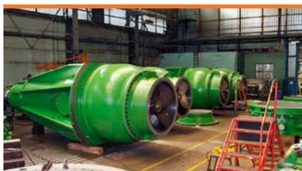
Axial and angular-flow single-stage semi-submersible with regulation system of hydraulic characteristics pumps
